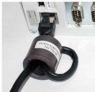
Fig.. 42 Ethernet cable, double loop through ferrite
