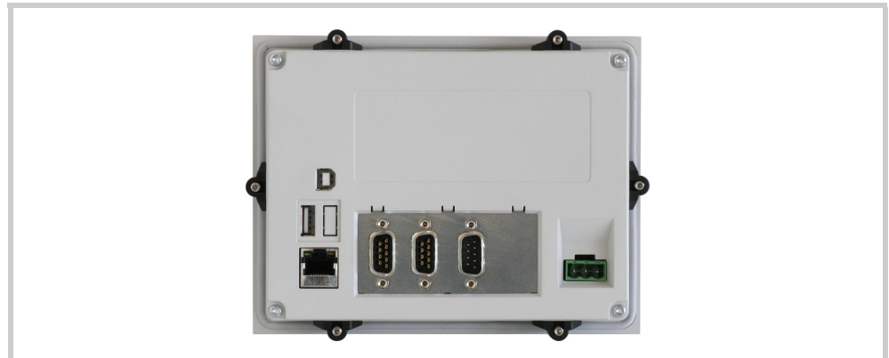
Fig.. 34 5.7" devices with six retaining brackets (meet IP65 / NEMA 4X requirements)
